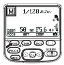
• Press the <MODE> button and set the flash mode to M.
